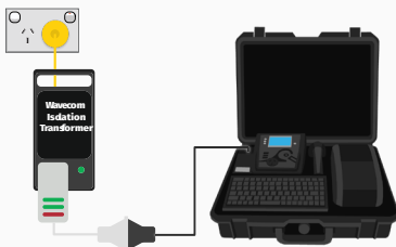
Testing Portable RCDs with no physical switch
